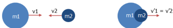
Figure 16.4. The nonelastic collision scheme between two particles. (Left) Before collision, (Right) after collision.
